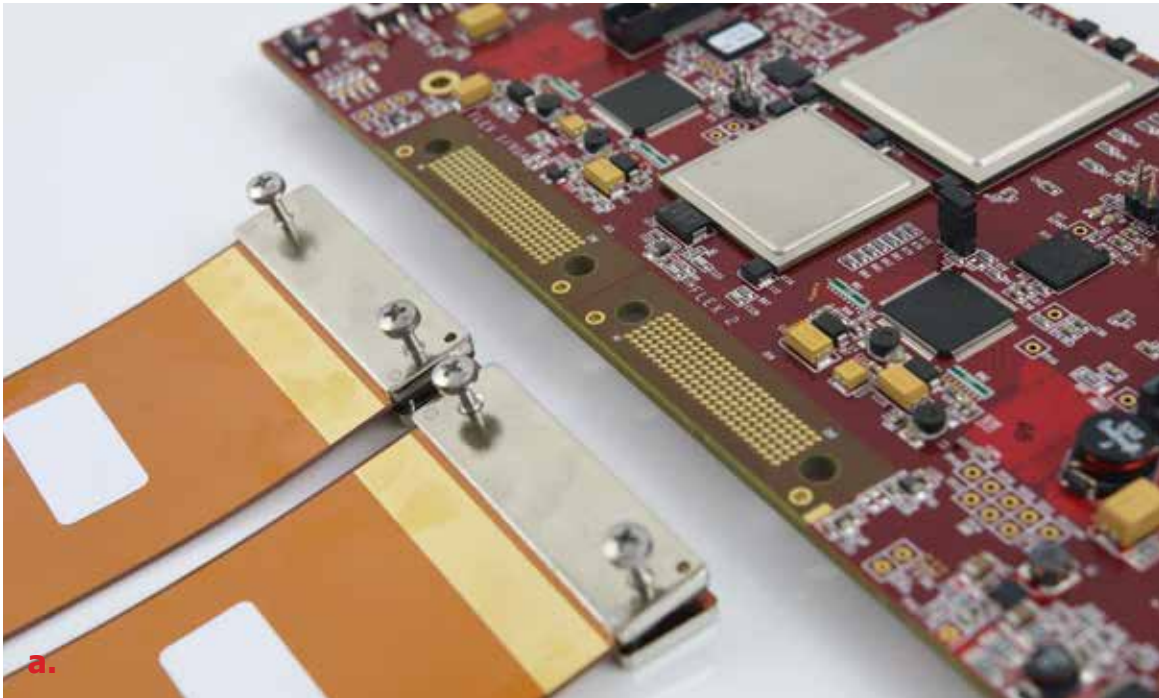
Figure 3-2. Connecting Flex Cable(s) to DMD Board
