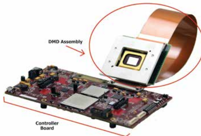
Figure 1-2. DLP Discovery 4100 .95" 1080p Development Kit
